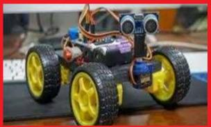
EXplore how ultrasonic and IR sensors detect obstacles and interface with microcontrollers.
