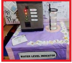
The Water Level Indicator is designed to monitor and display the water level in a tank, helping to prevent overflow and ensure efficient use of water resources.
